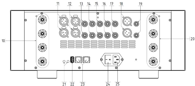
**10:** 2 speaker outputs, **right channel**. Connect the red socket to the positive terminal of the speaker, and the white socket to the negative terminal. The 4 sockets per channel allow you to use two cables per channel, one for the bass and one for the midrange (provided your speaker has a bi-wiring terminal). The two jacks marked red and white are connected in parallel, so it does not matter which one you use.
